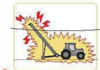
Be aware of overhead wires when moving equipment.
