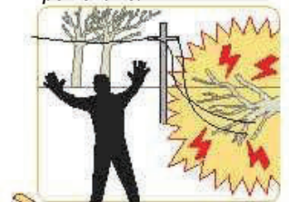
Stay 30 feet away and report fallen lines immediately.
